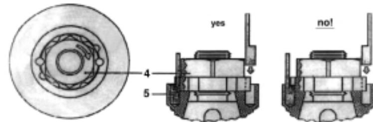
One thread can be exposed aft of either nut system, if more than that are showing it will be necessary to cut off the excess with a hack saw. If too many threads are exposed it will raise the central cone gear (6) and effect the performance of the propeller.
